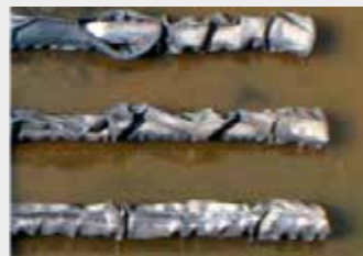
Fig. 2: Destroyed by chemical reaction with oil
